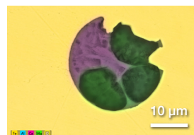
Figure 3. ColorSEM Technology image of the inclusion shown in Figure 2 in grayscale.
